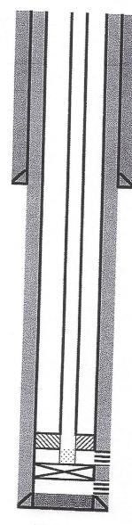
TD @ 4,000' PBTD @ 3,770' 12 1/4" hole 8-5/8" (24#) @ 1,550' w/ 775 sks, circ 121 sks TOC @ surf
