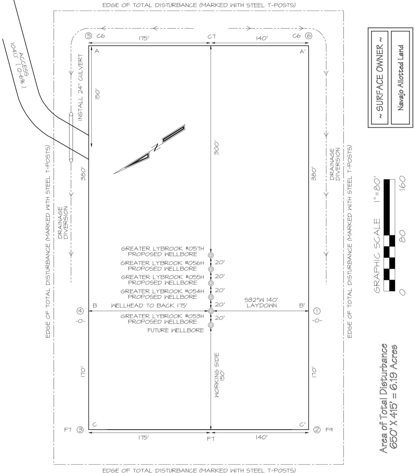
Steel T-Posts have been set to define Edge of Disturbance limits which are 50' offset from edge of wellpad.
