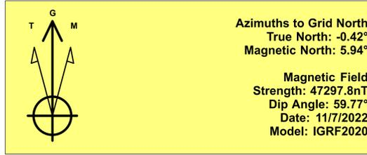
To convert a Magnetic Direction to a Grid Direction, Add 5.94°
