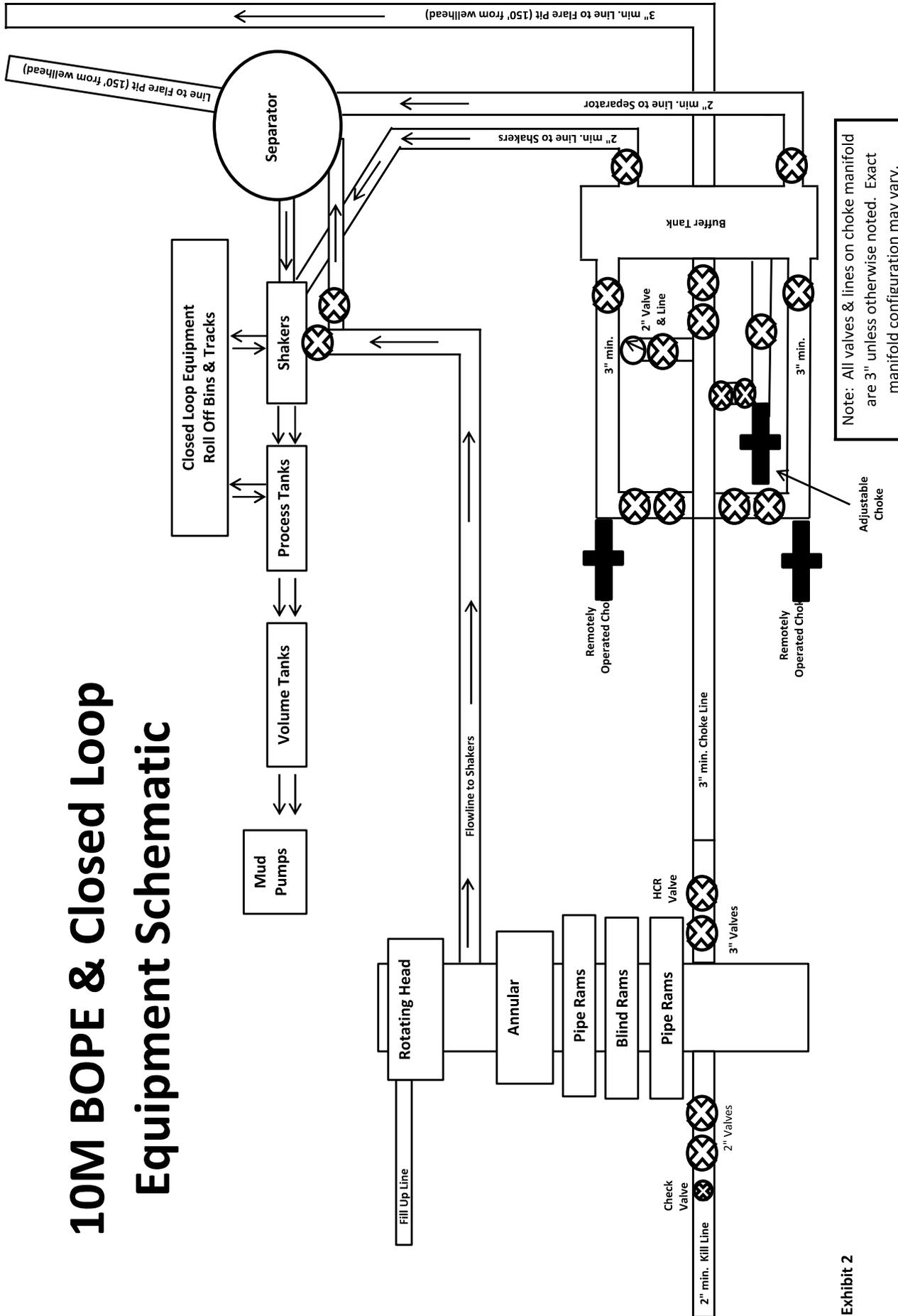
Note: All valves & lines on choke manifold are 3" unless otherwise noted. Exact manifold configuration may vary.
