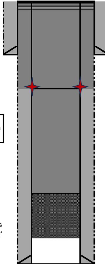
**Plug 3:** Top off plug. Cut off WH, top off casings and cellar as needed. Install P&A marker.
