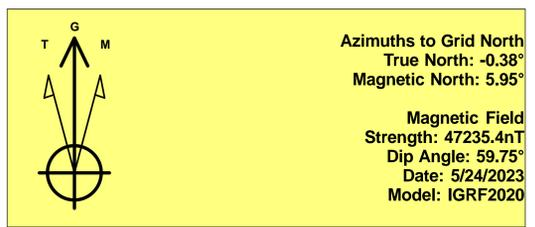
To convert a Magnetic Direction to a Grid Direction, Add 5.95°
