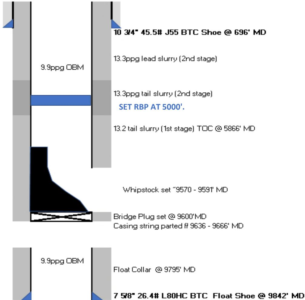
OXY PLANS TO TA THE WELLBORE SINCE WE WERE UNABLE TO SIDE TRACK FROM THE WHIPSTOCK. THE PROCEDURE WILL BE TO:
