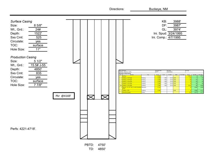
12/12/2022: PHW Wireline: RIH with 1.250" tool string with sample bailer tagged at 4570', recovered sample 3/14/2023 Scan and reject entire tbg inj string. Cleanout from 4,180'-4,750'. Replaced tbg string and RWTI.
