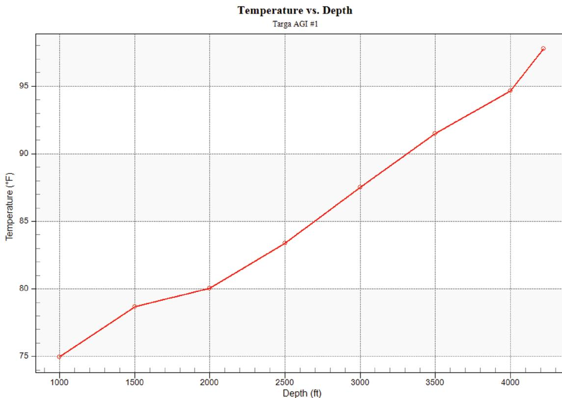
Figure 3. Initial pressure and temperature gradients measured prior to fluid injection test operations on April 18, 2023. Observed gradients for pressure and temperature are 0.4383 psi/ft. and 0.0071 F°/ft, respectively
