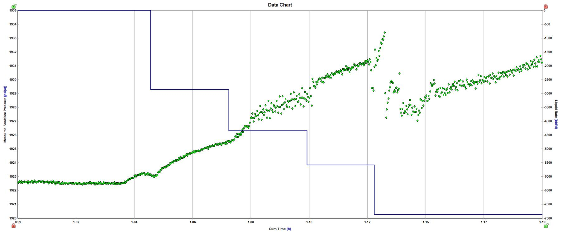
Figure 3: Depth-Corrected Sandface Pressures and Injection Rate Ramp-Up
