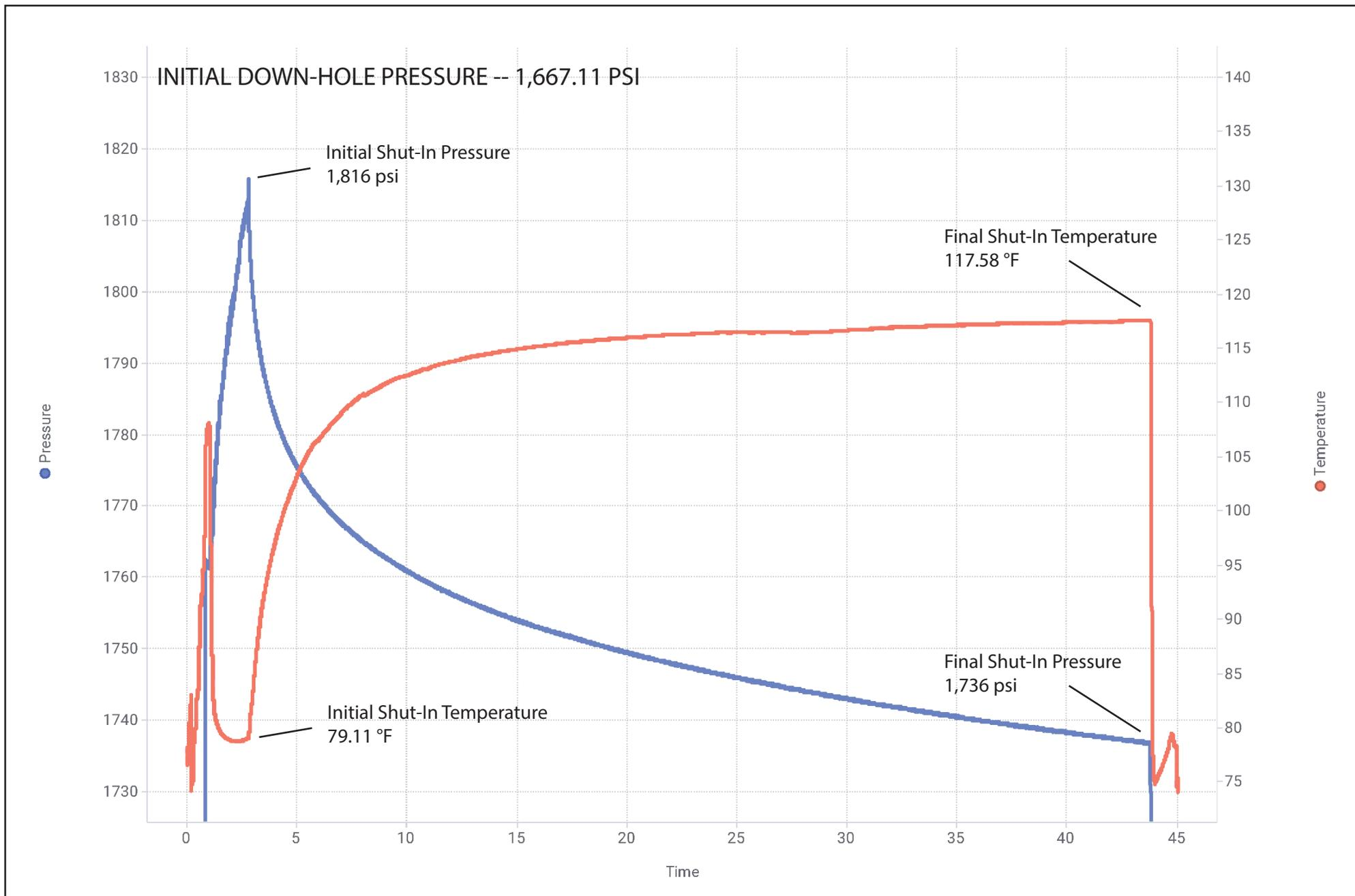
Figure 4. Recorded down-hole pressure and temperature trends during injection operations, and post-injection monitoring period (approximately 41 hours)
