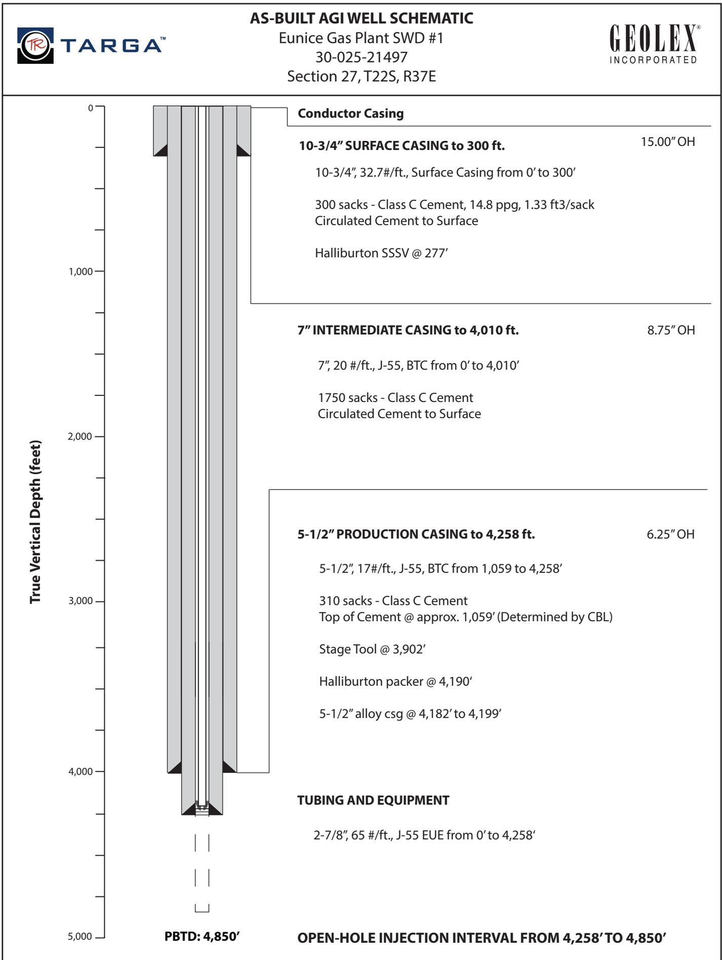
Figure 2. Eunice Gas Plant SWD #1 as-built well schematic
