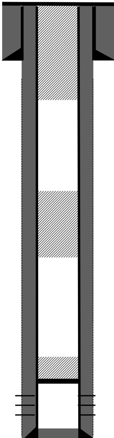
7" 20# casing @ 132'. Cemented with 65 sks Type 5 cement.
