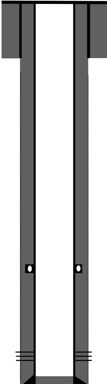
8-5/8" J-55 24# casing @ 210'. Cemented with 135 sks Class B (159 Cu.ft). Circulated 1.5 bbls cement to surface. Hole size: 12-1/4
