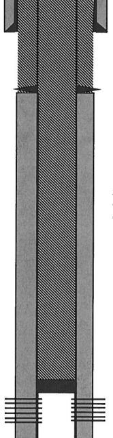
7" Surface Casing Set @ 21'. Cemented w/ 9 sks cement. Hole size 12-3/4"
