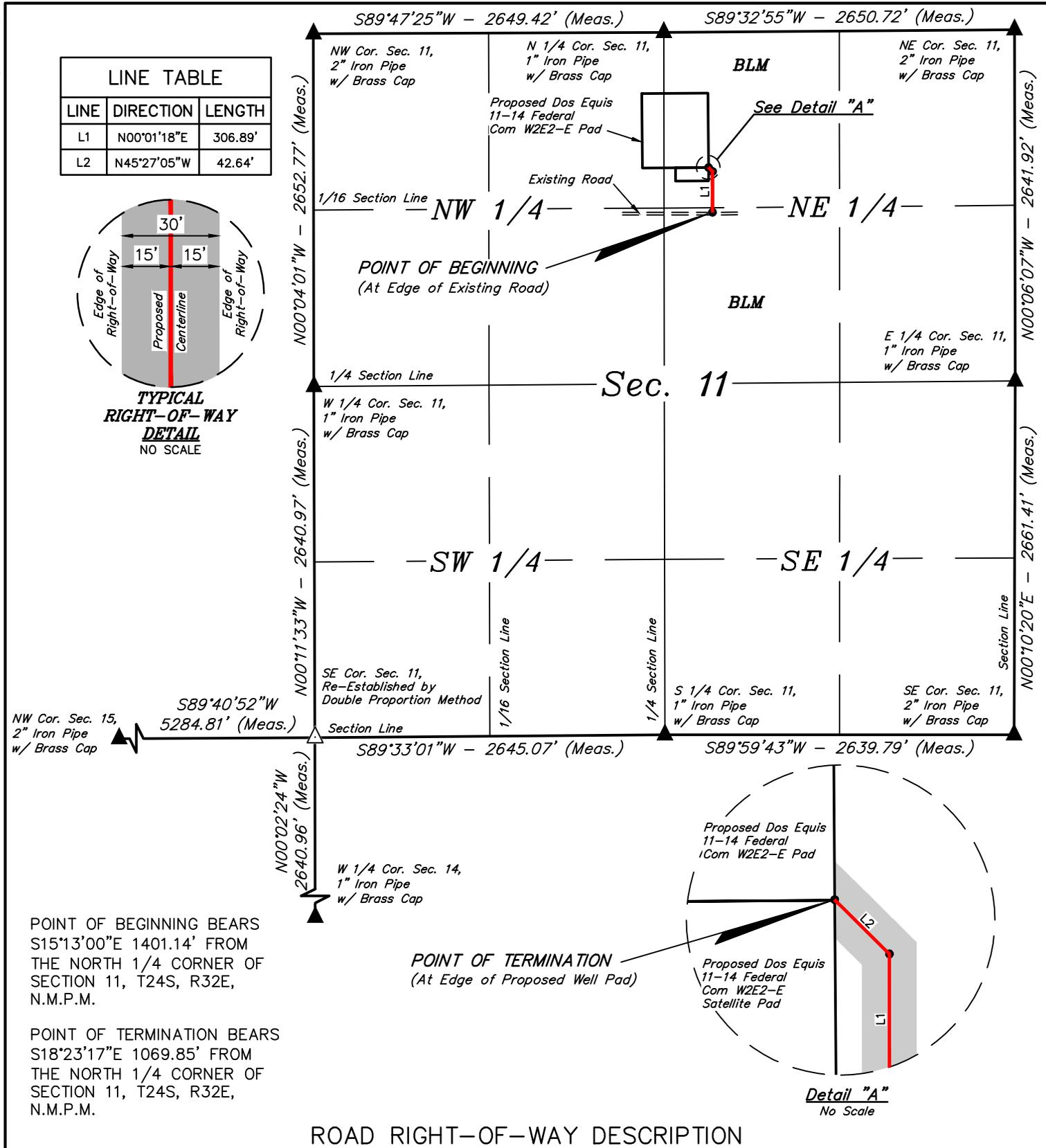
POINT OF BEGINNING BEARS S15°13'00"E 1401.14' FROM THE NORTH 1/4 CORNER OF SECTION 11, T24S, R32E, N.M.P.M.
