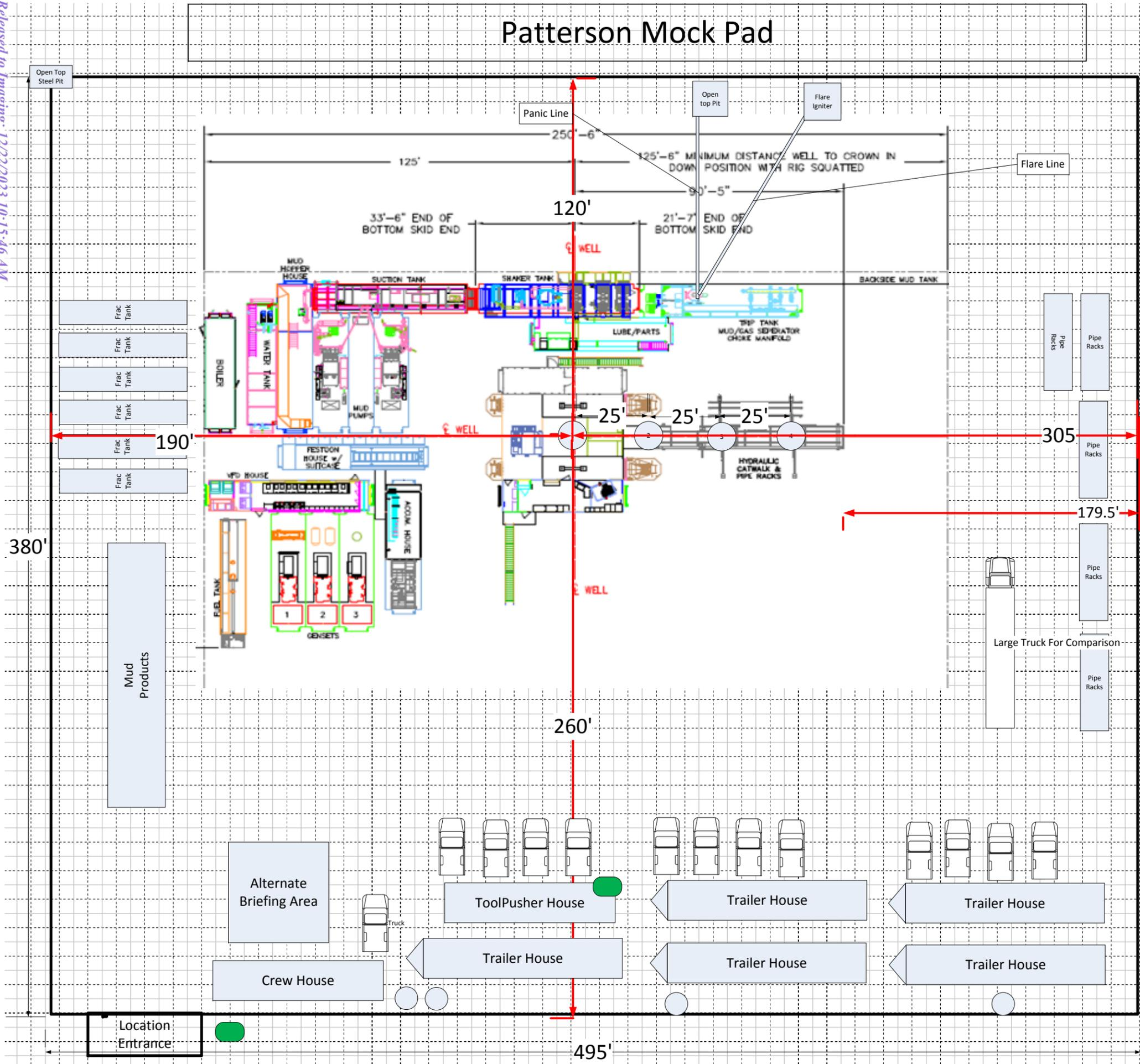
Rig layout shows rig in first and last well for illustration purposes.
