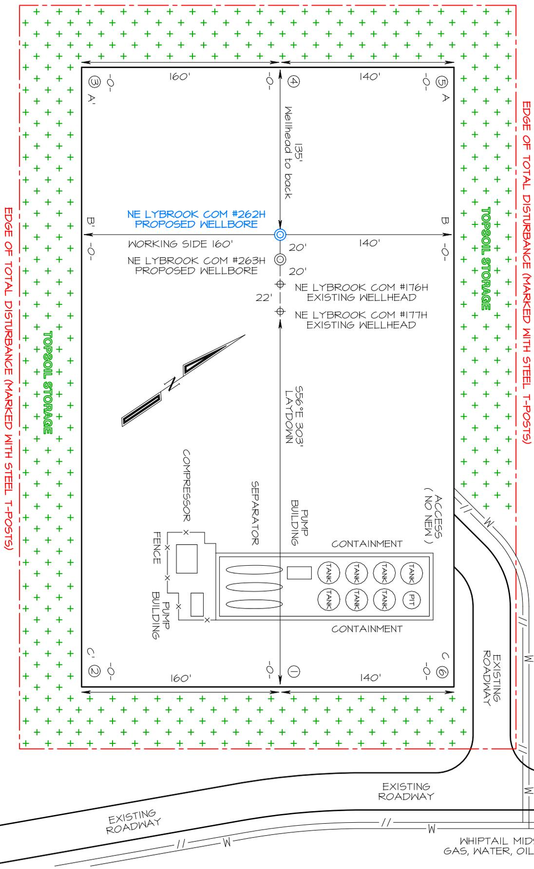
Steel T-Posts have been set to define the Edge of Disturbance limits which are 50' offset from the edge of the staked wellpad.
