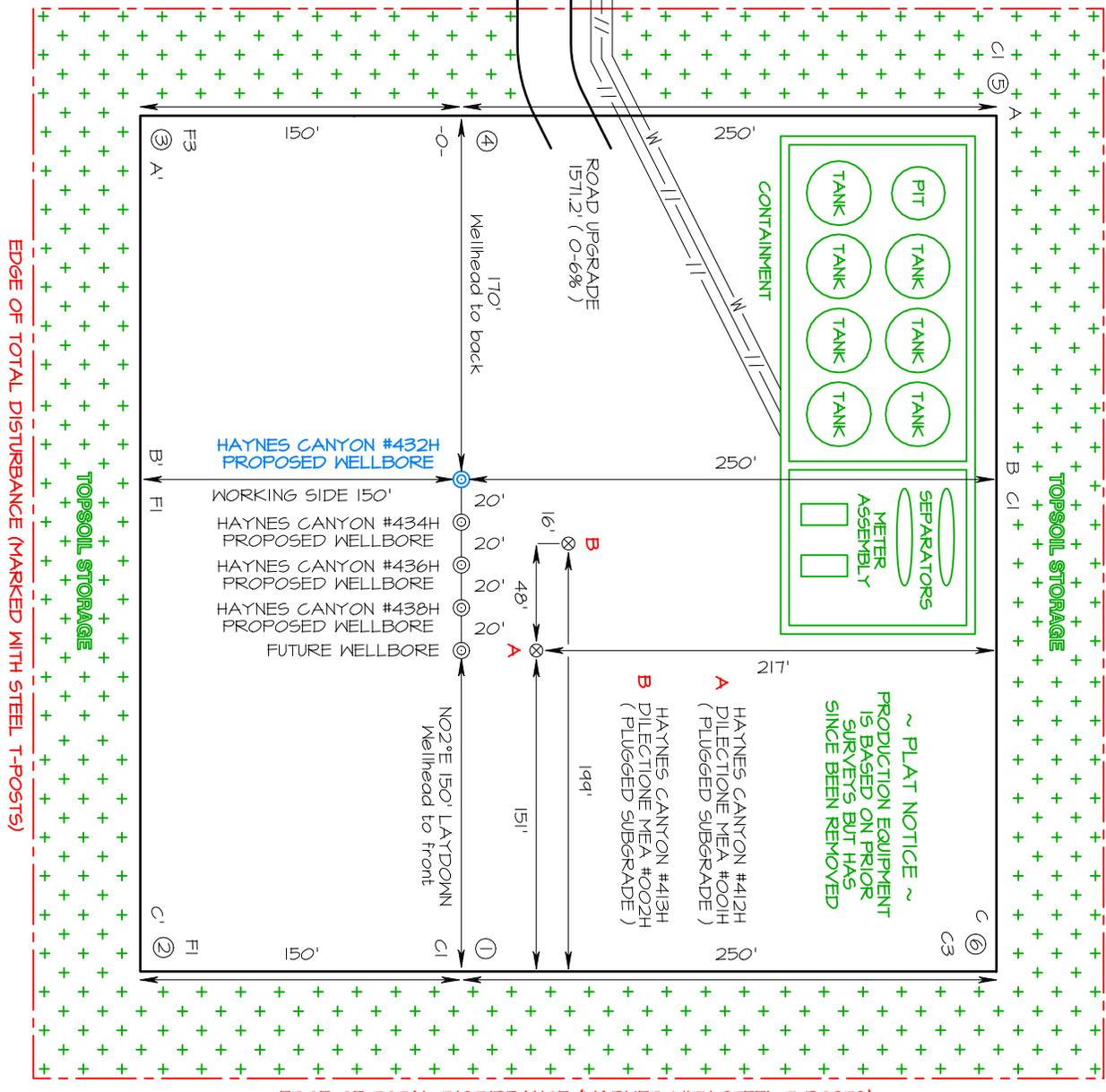
EDGE OF TOTAL DISTURBANCE (MARKED WITH STEEL T-POSTS)
