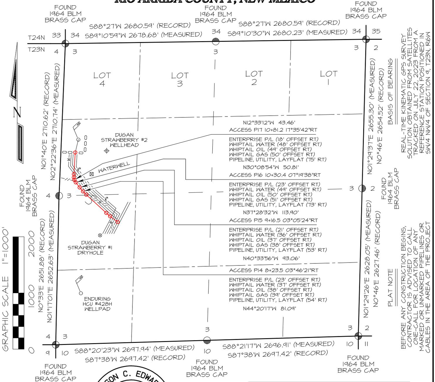
REAL-TIME KINEMATIC GPS SURVEY SOLUTION OBTAINED FROM SATELLITES TRACKED ON JULY 22, 2023 FROM A REFERENCE STATION POSITIONED IN SW/4 NW/4 OF SECTION 9, T23N, R6W
