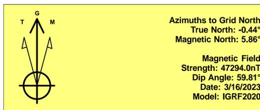
To convert a Magnetic Direction to a Grid Direction, Add 5.86°
