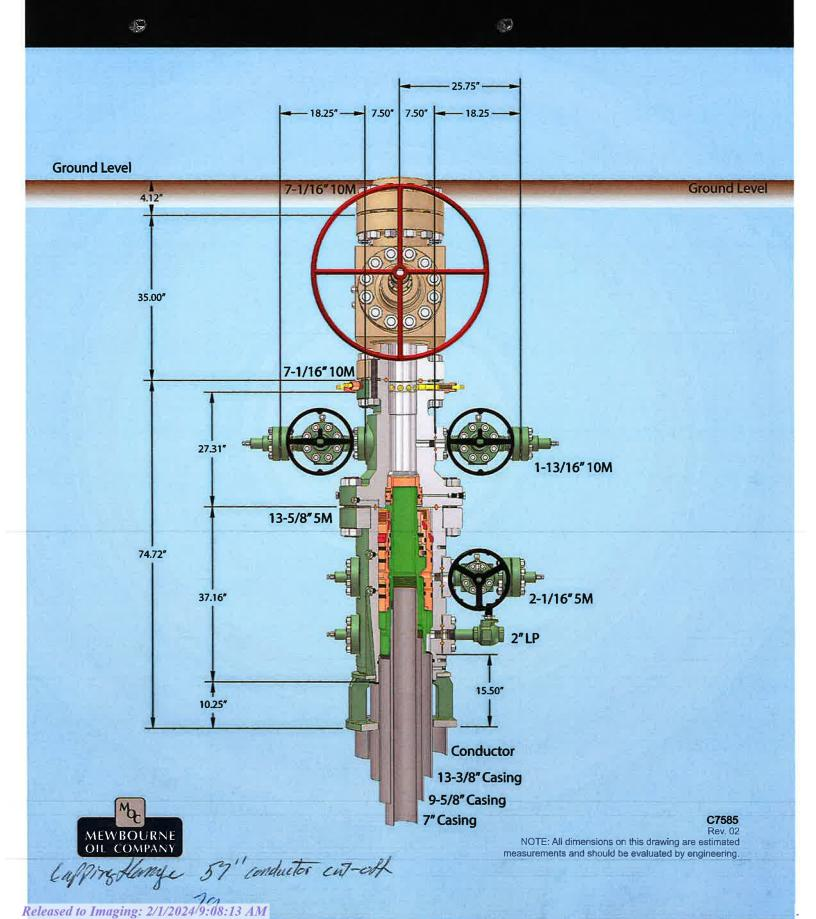
Sand Chute 4 B2AP Fed Com #1H Surface Csg
