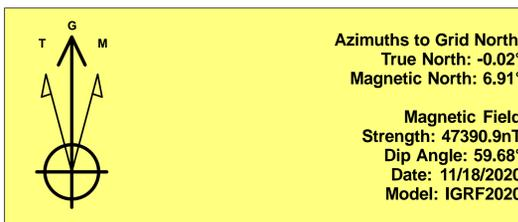
To convert a Magnetic Direction to a Grid Direction, Add 6.91°
