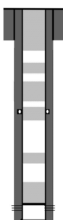
8-5/8" J-55 24# casing @ 320'. Cemented with 265 Cu.ft Class B. Circulated to surface
