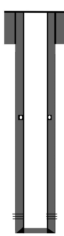
8-5/8" J-55 24# casing @ 320'. Cemented with 265 Cu.ft Class B. Circulated to surface
