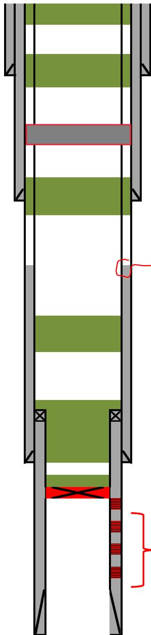
PERF & CIRC 60 SX CLASS "C" CMT @200'-0". TAG. (4HRS. CaCl) (SURFACE PLUG)
