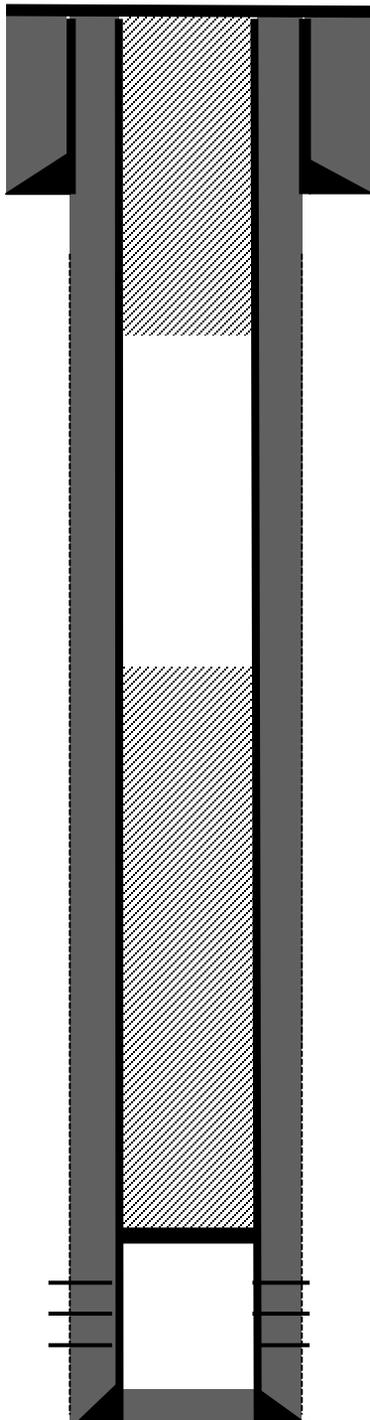
7" 23# casing @ 127'. Cemented with 50 sks, 59 Cu.ft Class B cement.
