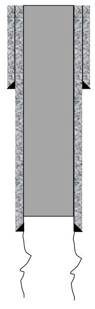
9-5/8" 28 # CASING SET @ 450' IN 12-1/4" HOLE. CEMENT CIRCULATED TO SURFACE W/150 Sks.
