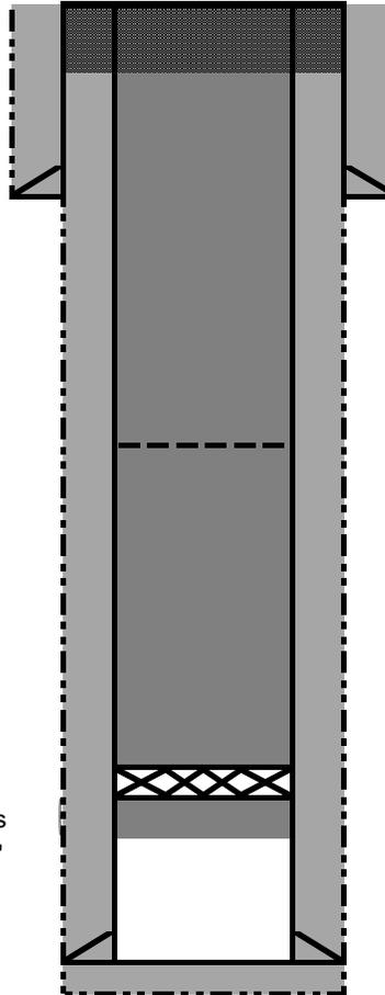
11-9-2023: Plug 4: Top off: Cut off WH, TOC at 100' in 7" and 4 1/2" casings. Install P&A marker. Mix and place plug of 46 sx via poly pipe to top off casings and cellar.
