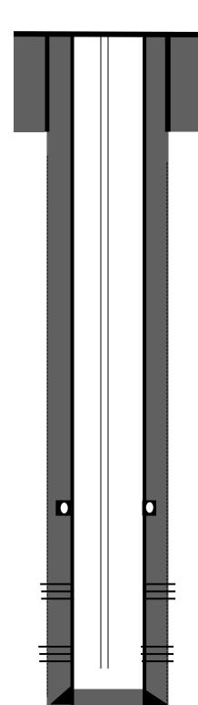
8-5/8" J-55 24# casing @ 205'. Cemented with 135 sks Class B. Circulated to surface
