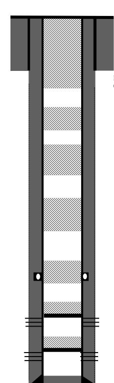
8-5/8" J-55 24# casing @ 205'. Cemented with 135 sks Class B. Circulated to surface
