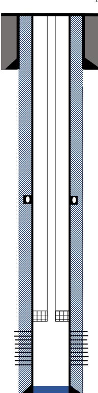
**Surface Casing:** 9-5/8", 36# J-55 casing set @ 346' **Cement Job**: 200 sks, Class G cement, 236 cu ft cement. Circulated 12 bbls to surface.
