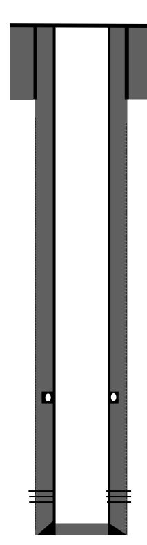
8-5/8" J-55 24# casing @ 206'. Cemented with 135 sks Class B. Circulated 2 bbls cement to surface
