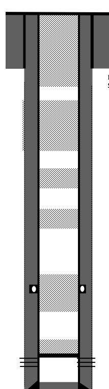
8-5/8" J-55 24# casing @ 206'. Cemented with 135 sks Class B. Circulated 2 bbls cement to surface
