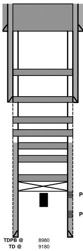
13 3/8 48# CSG @ 487 10. Perf'd @ 537'. Sqz'd 170 sx class C cmt @ 537' & circulated to surface.
