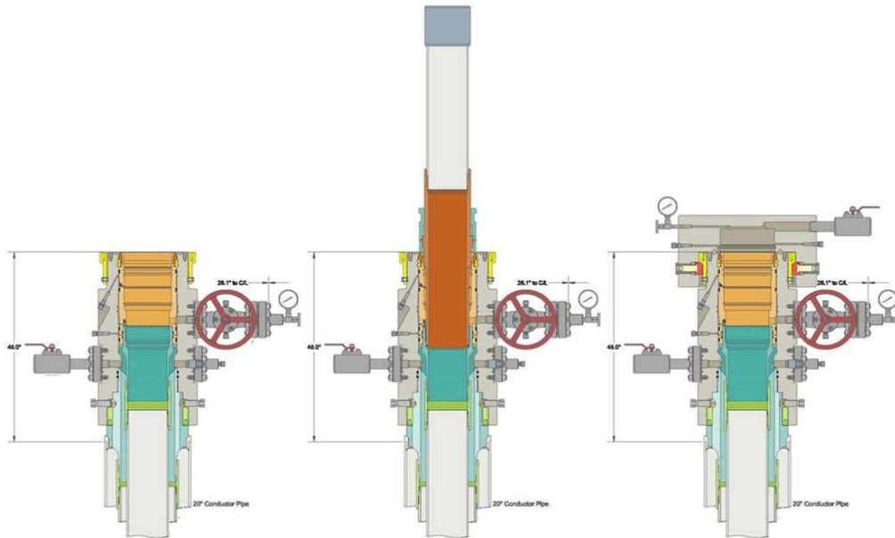
Intermediate 2 Casing – PR intends to Batch set all Intermediate 2 casing strings to a depth approved in the APD, typically set into Captain past losses. Appropriate notifications will be made prior Testing BOPE, and prior to running/cementing all casing strings.
