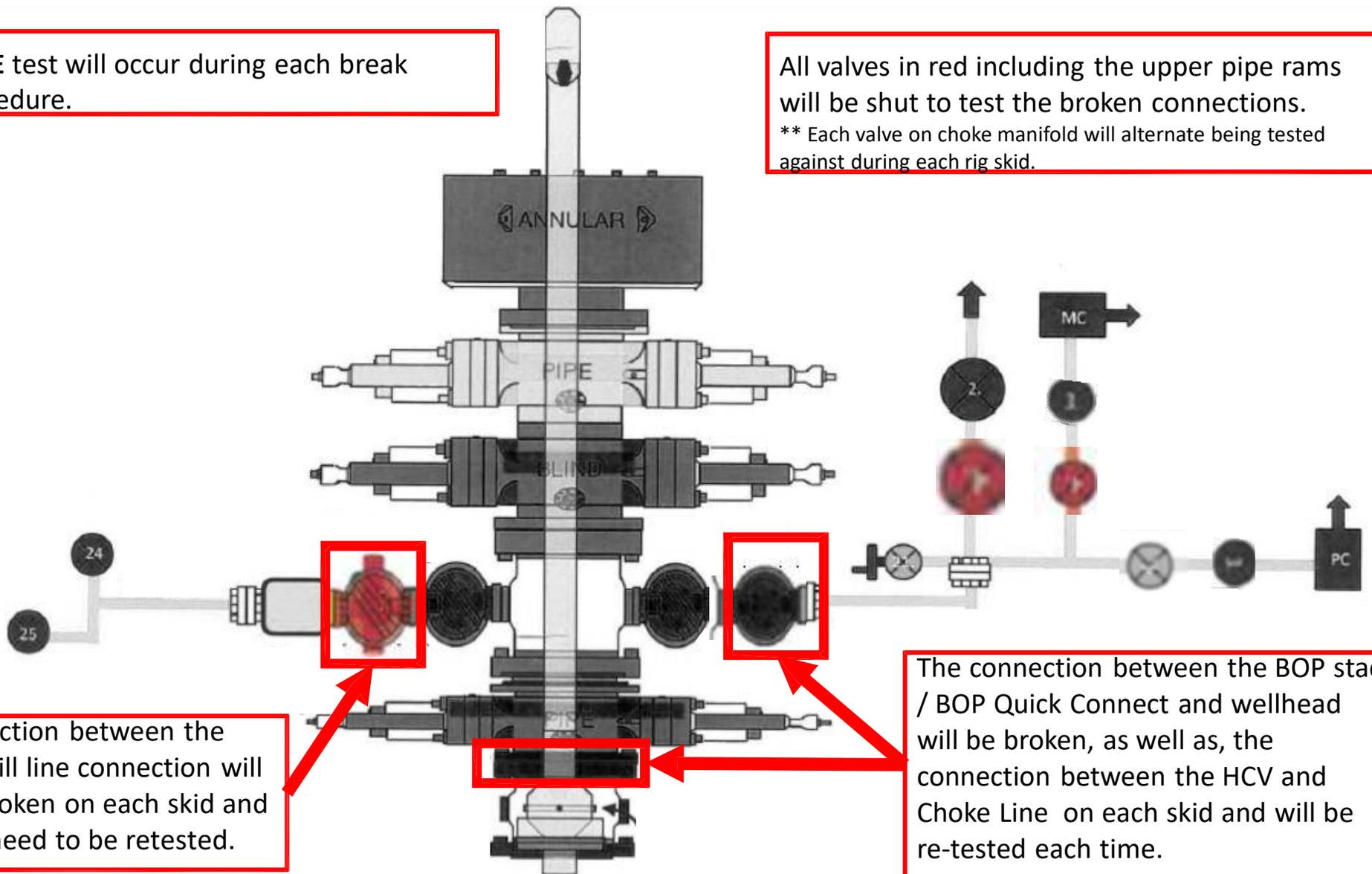
The connection between the HCV and kill line connection will **NOT** be broken on each skid and does not need to be retested.
