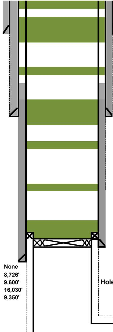
8. Perf & Circ 50 sx class "C" cmt from 100' - surface. ( Surface Plug)
