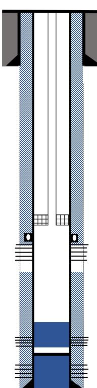
**Surface Casing:** 8-5/8", 24# casing set @ 294' **Cement Job**: 200 sks, Class B cement Circulated 75 sks cement to surface.
