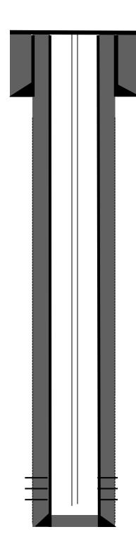
7" 20# casing @ 123'. Cemented with 89 cu.ft, Class B cement. Hole size: 9-1/8". Circulated 2 bbls cement to surface.
