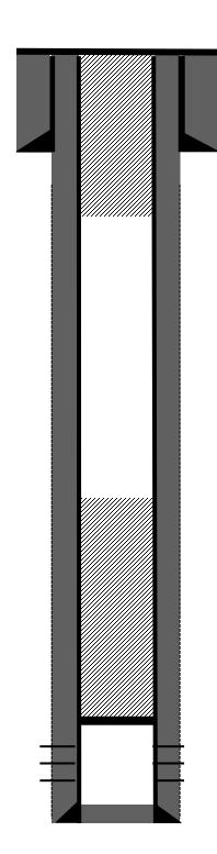
7" 20# casing @ 123'. Cemented with 89 cu.ft, Class B cement. Hole size: 9-1/8". Circulated 2 bbls cement to surface.
