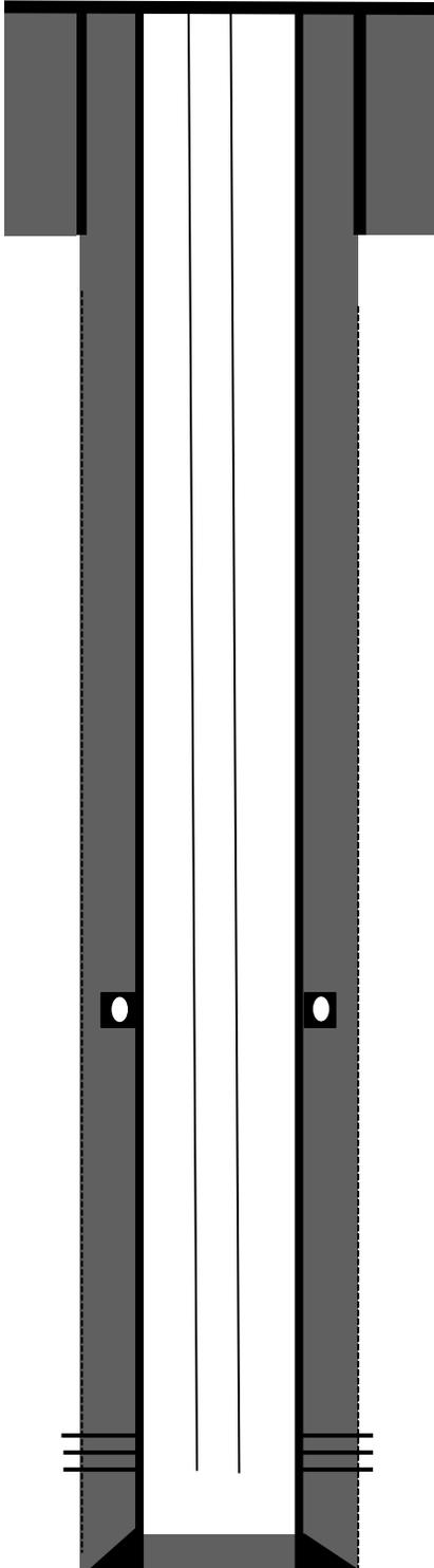
8-5/8" J-55 24# casing @ 277'. Cemented with 180 sks, 206.5 cf Class B w/ 3% CaCl<sub>2</sub>. Circulated 50 bbls to surface. Hole size: 12-1/4
