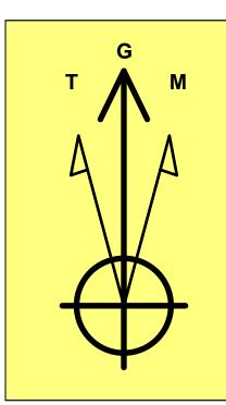
Azimuths to Grid North True North: -0.35° Magnetic North: 6.22°
