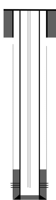
Cemented Stage 200 sks. TOC from temperature survey at 4620'.
