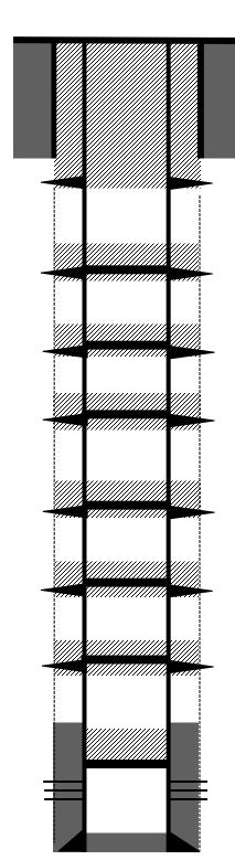
$10\,{}^{3}\!\!4"$  35.75# casing set at 215'. Cemented with 250 sks.
