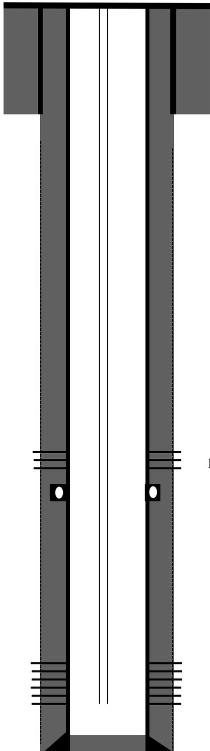
8-5/8" J-55 24# casing @ 293'. Cemented with 175 sks Cement.
