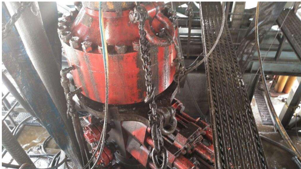
Figure 1: Winch System attached to BOP Stack
