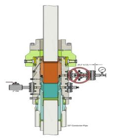
Run Intermediate Casing Land Intermediate Casing on Mandrel Hanger Cement Intermediate Casing Retrieve Running Tool
