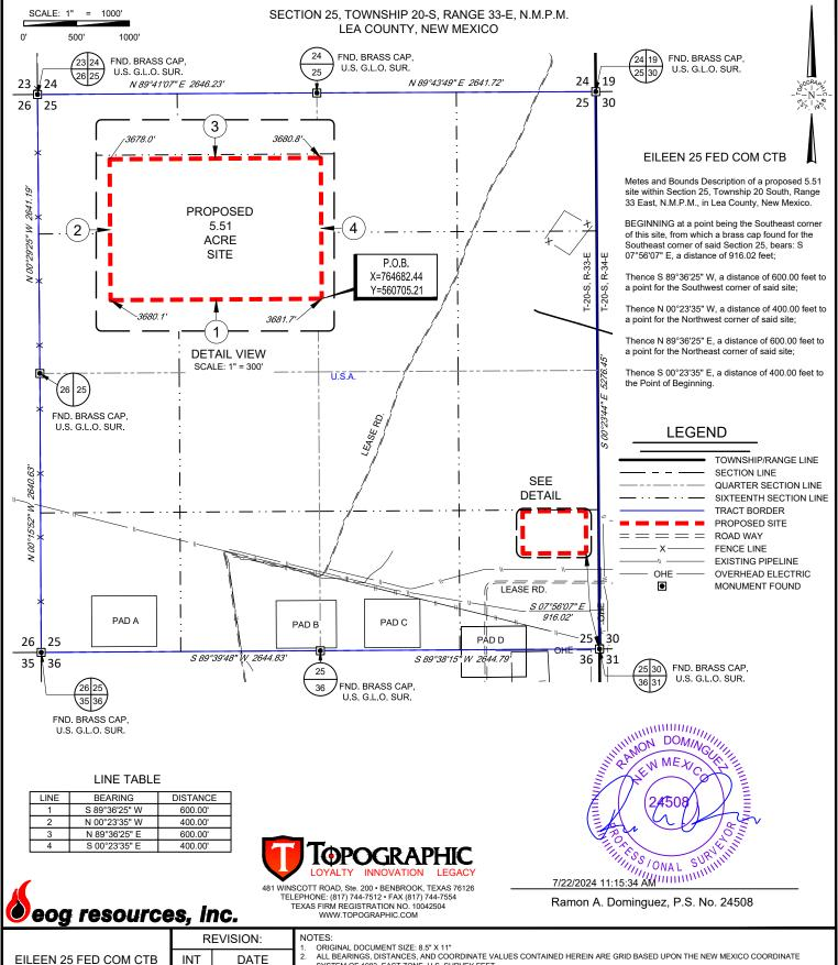
ORIGINAL DOCUMENT SIZE: 3,3 A 11 A 11 A 12 A 12 A 14 A 14 A 14 EARNINGS, DISTANCES, AND COORDINATE VALUES CONTAINED HEREIN ARE GRID BASED UPON THE NEW MEXICO COORDINATE SYSTEM OF 1983, EAST ZONE, U.S. SURVEY FEET.
