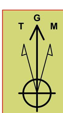
Azimuths to Grid North True North: -0.32° Magnetic North: 6.09°
