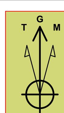
Azimuths to Grid North True North: -0.32° Magnetic North: 6.09°
