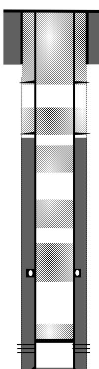
8-5/8" J-55 24# casing @ 198'. Cemented with 135 sks Class B (159 Cu.ft). Circulated cement to surface. Hole size: 12-1/4
