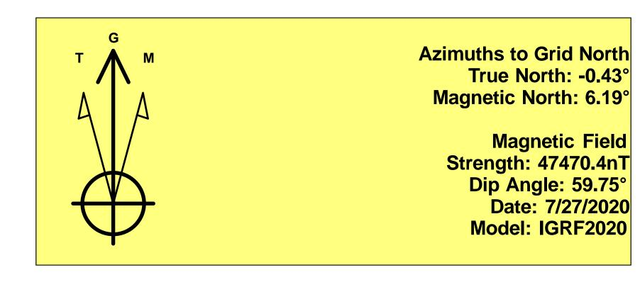
To convert a Magnetic Direction to a Grid Direction, Add 6.19° To convert a Magnetic Direction to a True Direction, Add 6.61° East To convert a True Direction to a Grid Direction, Subtract 0.43°
