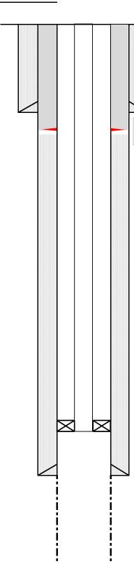
09/1992: Squeeze holes @ 1,727'. Cmt w/ 600 sx. Circ to sfc. Re-squeeze w/ 300 sx
