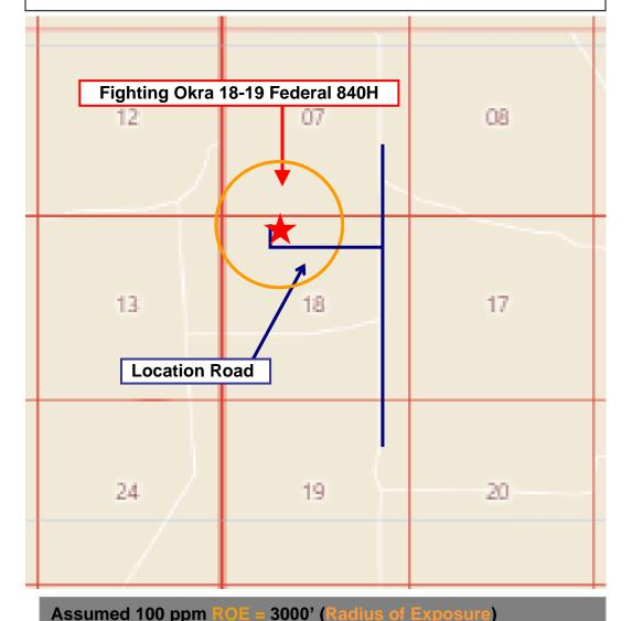
100 ppm H2S concentration shall trigger activation of this plan.
