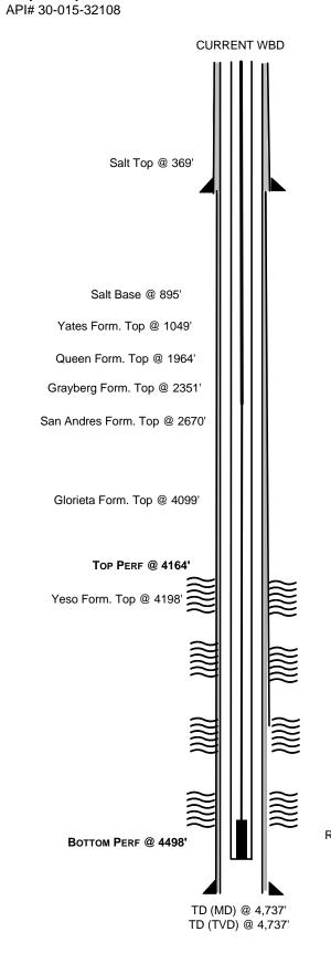
SURFACE 8-5/8" 24# J-55 Csg @ 403' CMT W/ 300 SXS P+2% CACL2 CIRCULATED 45 SXS TO SURF, TOC @ SURF
