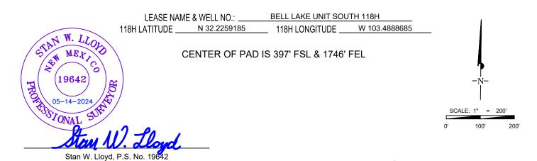
ALL BEARINGS, DISTANCES, AND COORDINATE VALUES CONTAINED HEREON ARE GRID BASED UPON THE NEW MEXICO COORDINATE SYSTEM OF 1983, EAST ZONE, U.S. SURVEY FEET. ELEVATIONS USED ARE NAVD88, OBTAINED THROUGH AN OPUS SOLUTION.
