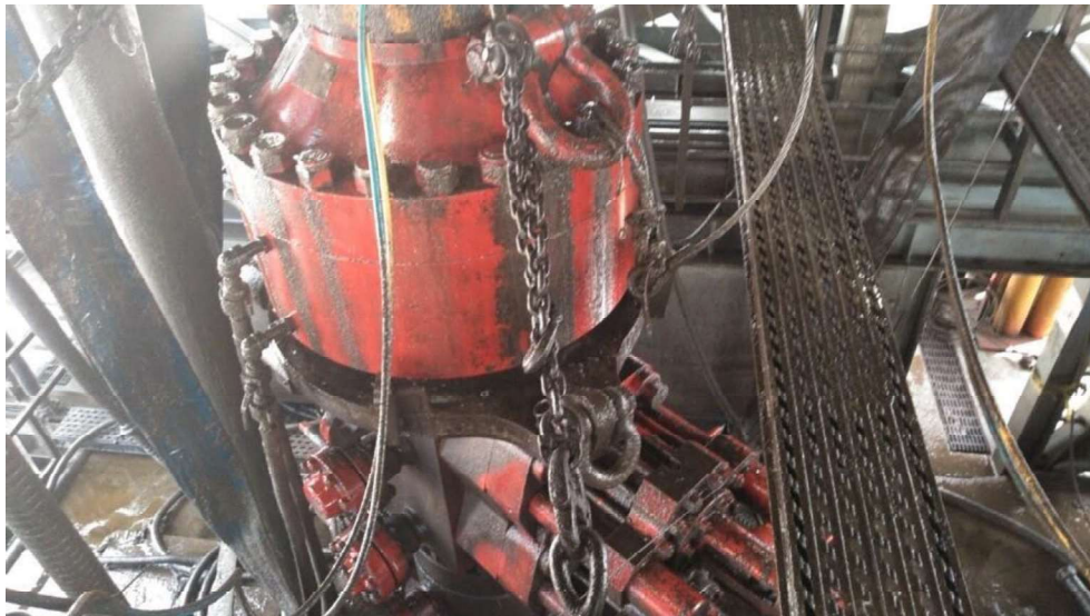
Figure 1: Winch System attached to BOP Stack
