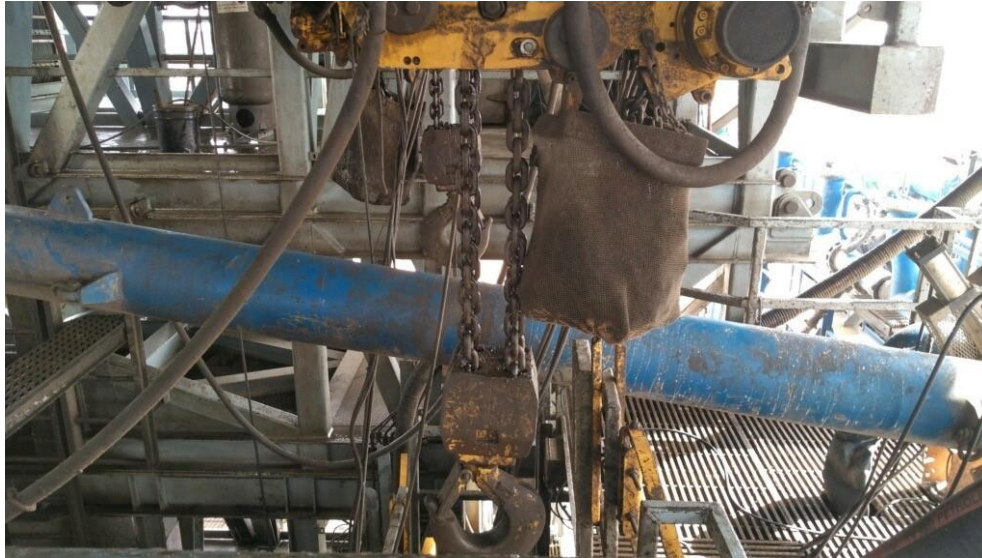
Figure 2: BOP Winch System
